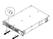
• Press and hold the black switch (see location designation below) to the right, while removing the power processing module.
