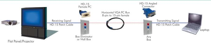
Application 5: 15 to 8-pin horizontal runs come directly from the wall/ceiling to connect to the viewing device.
