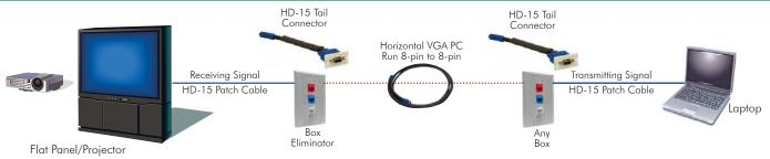
Application 4: 15 female to 8-pin horizontal run can be installed directly into the 1U VGA Module.
