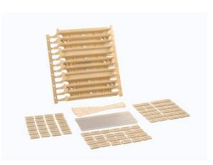
300-pair 110 Field Terminated Block Kit includes 300-pair 110 block with legs, 12 110C5 & 60 110C4 connecting blocks, and designation (110AB2-300 ft)
