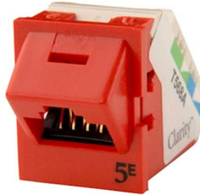
Clarity 5E Angled TracJack, ETL verified to TIA Category 5e component specification, is front-loading and front removable. New universal T568A/B wiring label and tapered wiring towers simplify termination. Center tuned to Clarity 5E patch cords for significant performance above Category 5e.
