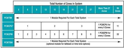
\*Note: One PCMPS2 Power Supply (not included) is required for each PCMCPU Module.
