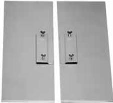
Helps prevent injury to workers by stabilizing floor-mount enclosures which are not bolted down. To install, slip the stabilizer under the floor stand and tighten two thumb screws. Made from .19-in. (5-mm) steel plate. Bright orange finish.
