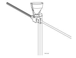
**3.18.** Lubricant should be applied according to the manufacturer's recommendations. Some lubricant vendors recommend an applicator to coat the cable as it enters the innerduct, others suggest distributing lubricant throughout the innerduct by pulling a swab through the innerduct as part of the pull-line placement. Pumps or gravity feed devices can also be used to inject lubricant into the innerduct.
