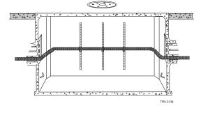
**5.25.** Store coiled splicing slack in the splicing manholes so that it is not likely to be damaged during later work in the manhole. If possible, store the slack in an enclosure designed to store splicing slack and a splice closure. Place an end cap on any bare cable ends to prevent moisture or dirt intrusion.
