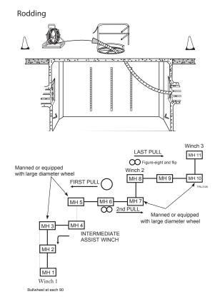
Inspect potential reel and winch locations for their suitability and make plans for installation techniques such as backfeeding or use of intermediate assist winches.
