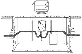
**5.26.** Fiber optic warning signs should be placed on all innerduct containing fiber optic cable. Warning signs can help prevent damage resulting from the cable being mistaken for something else.
