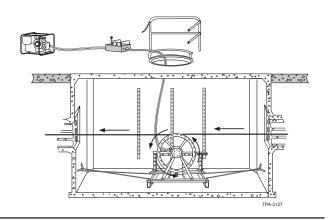
**4.3.** Use of multiple winches requires compatible pulling equipment and careful coordination of winch speeds. Consult the equipment manufacturer's instructions for necessary details.
