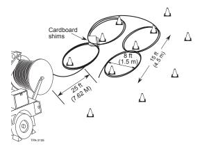
Traffic cones spaced 7-8 feet apart are useful as guides during figure-eighting. When figure-eighting long lengths of cable, care should be taken to relieve pressure on the cable at the crossover of the eight. This can be done by placing cardboard shims at the crossover or by forming a second figure-eight.
