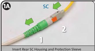
nsert Rear SC Housing and Protection Sleeve onto the Field Fiber. Proceed to Step 2
