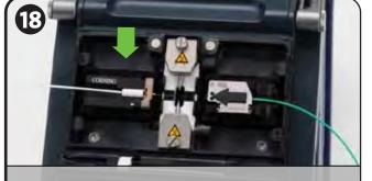
Load the Connector Holder into the Splicer (on the Left Side)
