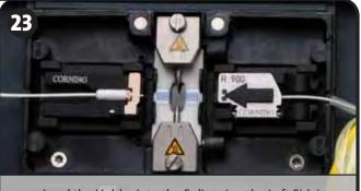
Load the Holder into the Splicer (on the Left Side)
