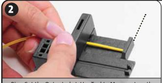
Ring Cut the Outer Jacket; Use Tool to Measure Length Remove Jacket
