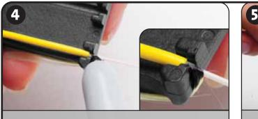
Mark the 900  $\mu m$  Fiber at Edge of Tool for Stripping
