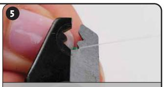
Strip the 250 µm Coating with the Smaller Notch
