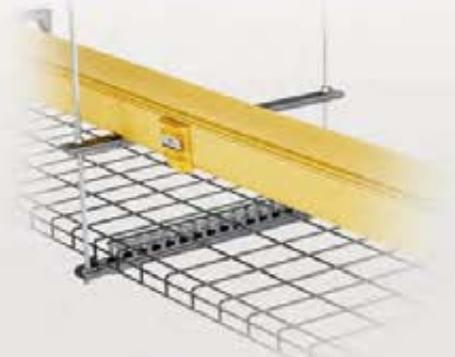
Brackets allow FiberRunner® 4x4, 6x4, 12x4 and 24x4 Pathways to be supported at any height above or below the Wyr-Grid® System. This installation utilizes the same threaded rod to support both systems.
