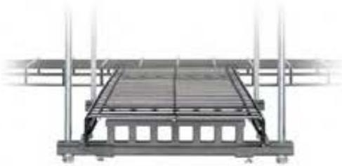
Trapeze brackets are supplied with integral slide clips for securing the pathway in place, eliminating loose hardware. In addition, trapeze bracket design allows side to side pathway positioning increasing installation adjustability.
