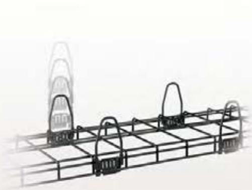
Optional snap-on sidewalls require no hardware or tools for installation. The sidewalls are available in three heights: 2" (50mm), 4" (102mm), and 6" (152mm).
