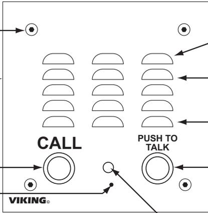
**Microphone:** Omni-directional microphone with protective water-resistant cloth.
