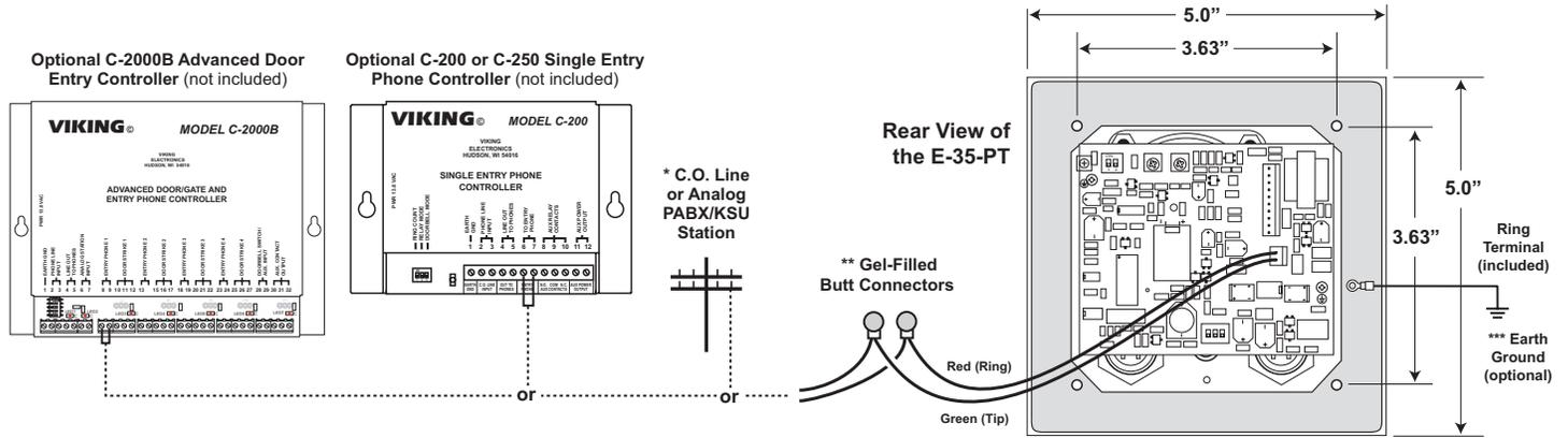
\* **Note:** When installing a line powered phone on a low voltage and/or low loop current phone system extension, a **TBB-1B** Talk Battery Booster may be required, see **DOD# 632**.
