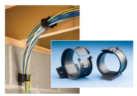
The CADDY® CATCR50 Cable Retainer is a plastic, low-voltage cable support with an easy-lock closure and an attachment base. The new cable retainer from ERICO® can be installed on walls, beams, studs, ceilings and racks – vertically or horizontally – which makes it extremely versatile. It is also suitable for airhandling spaces (plenum rating). The CADDY CATCR50 support has rounded edges to avoid over-bending and kinking of cables.
