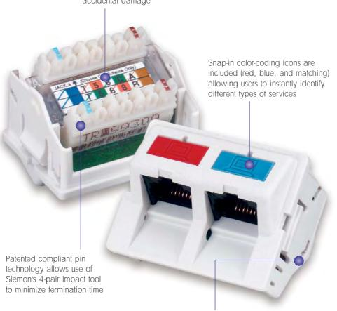
Cable-tie anchor points provide effective strain relief for cables entering from top or bottom of coupler
