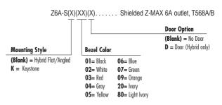
Outlet terminates S/FTP, F/FTP and F/UTP cable constructions with 22-26 AWG (0.64 – 0.51mm) solid and 26 AWG (0.48mm) stranded conductors, with up to 0.60mm diameter conductors and up to 1.48mm diameter over insulation.
