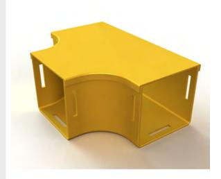
Horizontal Tees are used to branch off the main route or provide a method of breaking into horizontal duct. Standard tees branch off at the same size as the through duct. Transition tees branch off to a smaller duct. They are available with and without covers.
