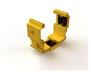
Joiners are used to connect the straight duct and components together. Simply snap the joiner into the slots at the end of each part to be joined. For straight duct that has been cut to length, new slots will need to be made with the proper slotting tool. "Slotless" joiners are available in sizes from 4" X 4" upwards that will join the fittings to the duct with or without joining slots.
