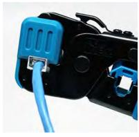
5) Terminate the plug with a modular plug crimper. Use the RJ45 8-position 8-contact cavity.
