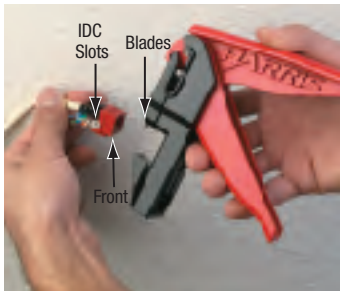
3. Insert jack in JackRapid front first with IDC slots facing blades of JackRapid.
