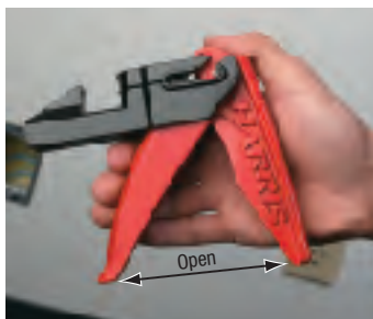
3. Make sure handle is open. Once pin #1 has been inserted, slide pin #2 into blade head.
