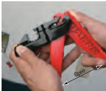
1. Make sure handle is in open position. Push handle and blade toward each other.
