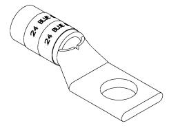
WIRE SIZE: # 6 AWG MATERIAL: HIGH CONDUCTIVITY COPPER FINISH: TIN PLATED
