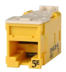
Clarity 5E High Density Jack, ETL verified to TIA Category 5e component specification. Rear-loading, 180° exit, 8 position. Quick and easy lacing cap termination. Universal T568A/B wiring label. Center tuned to Clarity 5E patch cords for optimum performance.
